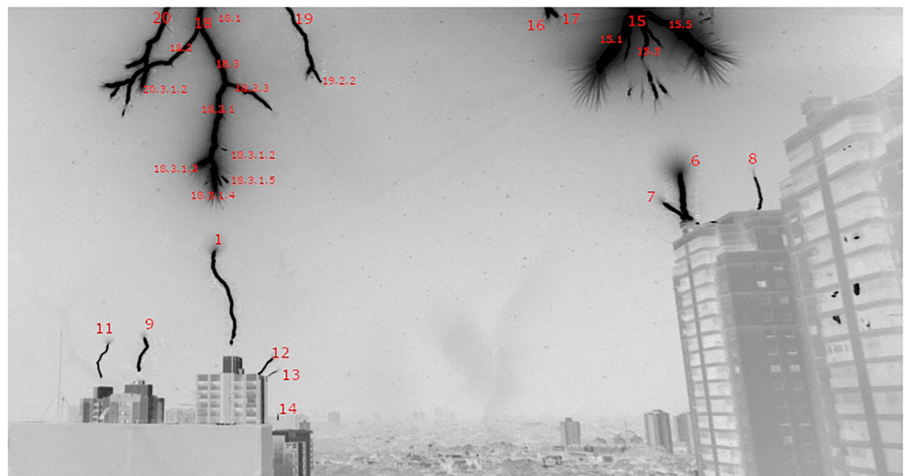
Figure 2. Lightning attachment to building 11. This figure shows one frame before the occurrence of the return stroke.
